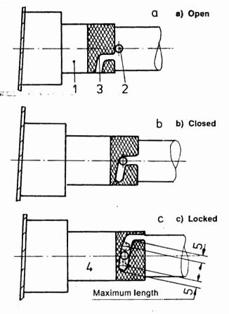
After connecting the quick lock couplings make a visual check that the collar is extended forward over the bearing far enough for the safety pin to engage. Having engaged the quick locks check that the safety pin cannot be moved without pressing it down. If it cannot be slid without pressing down the controls are properly connected.
